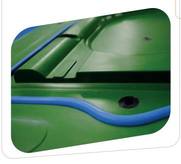
The mould is built with double seals; an outer vacuum seal and an inner resin seal. The flange area between the seals is evacuated to provide the main clamping force. This double seal also provides excellent security against vacuum leaks through the seals.
