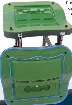
Due to the use of vacuum to provide a uniform clamping force, the VRTM process can be successfully used to mould large structures using relatively simple and low-mass tooling.
